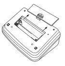
Remove the battery cover at mainframe and replace the four pieces of batteries.
